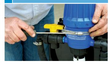
d Fix the suction hose of the Dosatron® to the valve under the tank. Cut the length of the suction hose (if necessary) to eliminate any loop in the hose (this will prevent the stagnation of the liquid).
