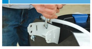
C Secure the installation of the **Dosatron® pump** on the tank support (b) with a clamp.
