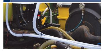
If desired: add a 2-way switch to be able to turn the mixer off and on, install a 12-volt electrical wire from the tractor to the electrical motor of the mixer. Make sure that the motor runs at all times when using the AGTIV® Liquid Injection kit.
