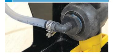
Select the right reducing nipple size to connect the **Main flow hose** ① from the existing in-furrow system to the AGTIV® Liquid Injection Kit & to the outlet ②.
