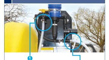
one from the flow meter coming from the existing in-furrow system to the main yellow valve of the injection kit.
